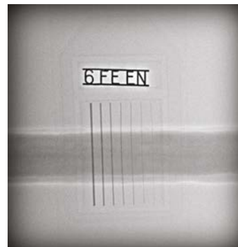
Still image. Accumulation 1 second. Wall thickness 18 mm.
