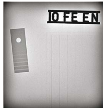
Still image. Accumulation 30 seconds. Wall thickness 40 mm. Contrast sensitivity 0.4%
