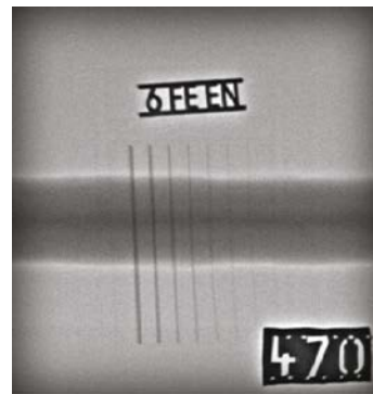
Pipe speed 4 m/min. Wall thickness 17 mm with 5 mm weld reinforcement. Contrast sensitivity 1%
